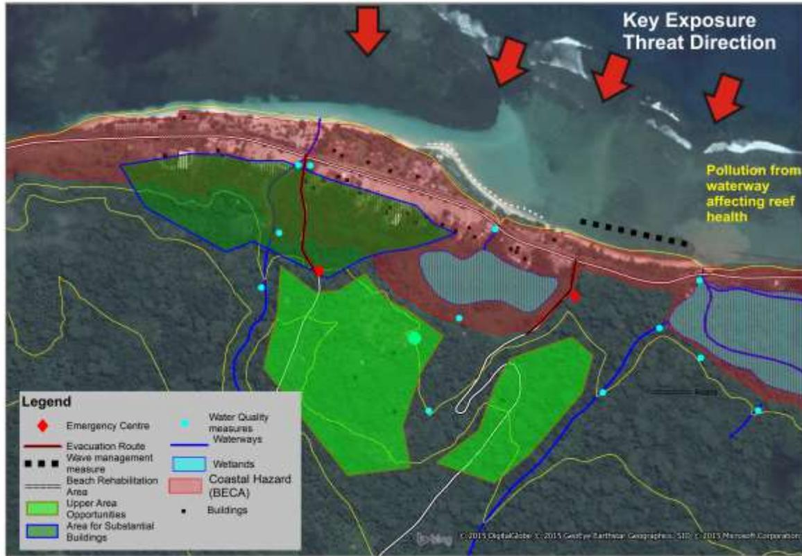
Figure 1 Overview of Structural Management Plan Options for Manase
